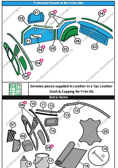
Denotes pieces that can be skived / thinned if ordered in Leather. Skiving is a process of thinning leather to make it more pliable without weakening it, making it easier for trimming round corners and curves.
