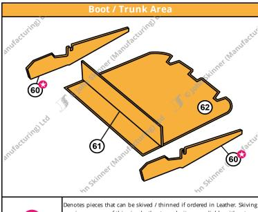
is a process of thinning leather to make it more pliable without weakening it, making it easier for trimming round corners and curves. This gives a neat & high quality finish.
